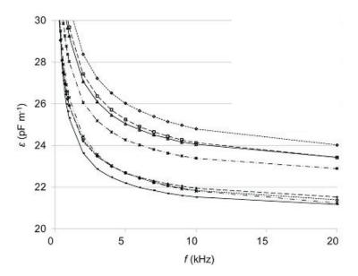
**Fig. 2.** Effect of electromagnetic field frequency, f, on the permittivity of the tested mixtures of wheat flour and oat meal. Explanations as in Fig. 1.
