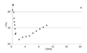
**Fig. 3.** Sums of relative differences in the dielectric loss factor between analyzed samples of tested material within the electromagnetic field frequency range of 100 Hz-20 kHz.
