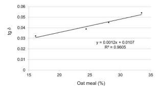
**Fig. 5.** Correlation between yield of wet gluten and the dielectric loss factor, tg  $\delta$ , of wheat flour and its mixtures with oat meal (f = 20 kHz).
