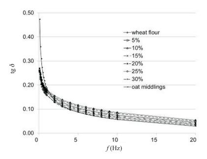
**Fig. 1.** Effect of electromagnetic field frequency, f, on the dielectric loss factor,  $\operatorname{tg} \delta$ , of the tested mixtures of wheat flour and oat meal.
