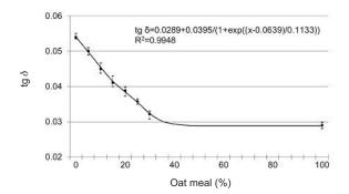
**Fig. 4.** Value of dielectric loss factor,  $\operatorname{tg} \delta$ , for tested mixtures of wheat flour with oat meal (f = 20 kHz).
