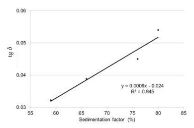
**Fig. 6.** Correlation between sedimentation factor and the dielectric loss factor,  $tg \delta$ , of wheat flour and its mixtures with oat meal (f = 20 kHz).
